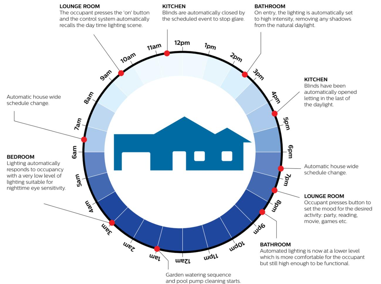
Rather than having multiple buttons for the same area to recall different lighting scenes – for example in the master bedroom, 'Morning', 'Afternoon', 'Evening' & 'Night' – a single button on a Dynalite user interface can be programmed so that the right scene is recalled for that specific time of day. This allows for a simplified experience with fewer buttons required.
