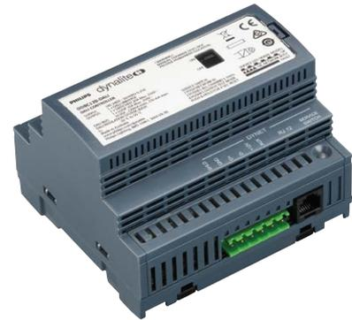
**Inbuilt diagnostic functionality** – Features lamp and driver failure reporting, driver run time tracking for each driver, emergency test reporting and device/driver online/offline status indication.
