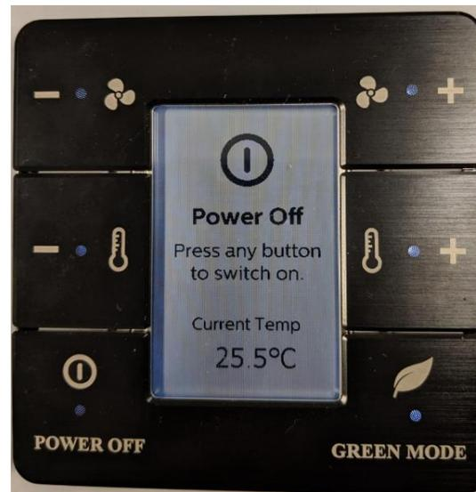
Showing the HVAC system response to balcony door or room window being open toggle the third switch from closed to open and the display will change its image to the example shown.
